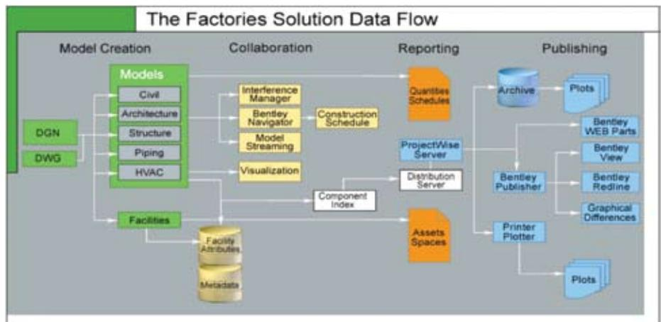
Figure 3: How Bentley supports the data workflow in the factory-planning process.
